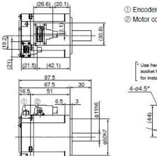
① Encoder connector ② Motor connector
